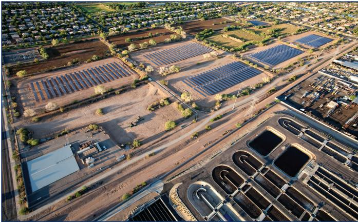
**Gilbert's Neely Wastewater Treatment Plant (11MGD)** solar at 2.2 MW mounted panels in the facility's recharge basin and adjusted panel height accordingly. Gilbert received a rate of \$.075/kWh with a 2.5% annual escalator and utility incentives. Gilbert's Wastewater Manager Mark Horn indicates savings close to \$2M were initially projected. He expects most savings to occur in the last 10 years of their contract but that "will depend on future utility rate increases."
