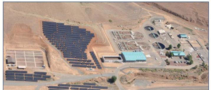
**Prescott Valley's Tank Farm and Booster Station's two solar systems (695 kW)** provide 50% of the power demand for the facility. The Town's **Advanced Wastewater Treatment Plant (2.6MGD)** two solar systems ( 765 kW) provide 30% of demand. Prescott Valley's solar footprint is 1.460 MW. Projects completed in April 2012 and
